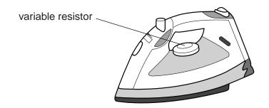
She uses the variable resistor in the iron to change the current.
