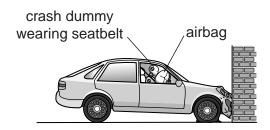
(a) When the car hits the wall, a sensor triggers the fast release of a large amount of gas into the airbag.
