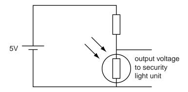
Explain how the potential divider circuit and the LDR can be used to turn on the security light when it becomes dark.
