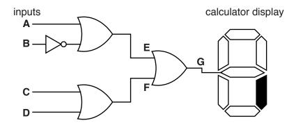
He completes part of the truth table. The output from the logic system switches the shaded segment on the calculator display on and off.
