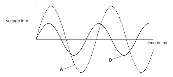
Graph  ${\bf A}$  shows the output from this small AC generator.
