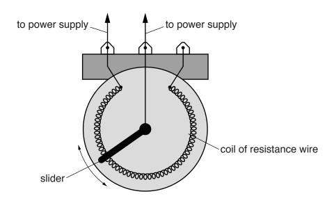
The slider moves around and keeps in contact with the coil of resistance wire.
