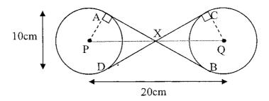
The points A, B, C and D above are the points at which the contact between the belt and the disc is lost.
